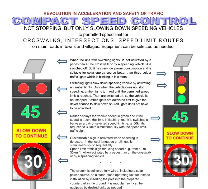
The intersection is normally uncontrolled so the traffic lights are turned off. Vehicles on the main road have priority. A pedestrian activates the compact crosswalk signalling and in the same time the speed limit sign 30 to slow down vehicles. It works as the uncontrolled crosswalk (see other side).
